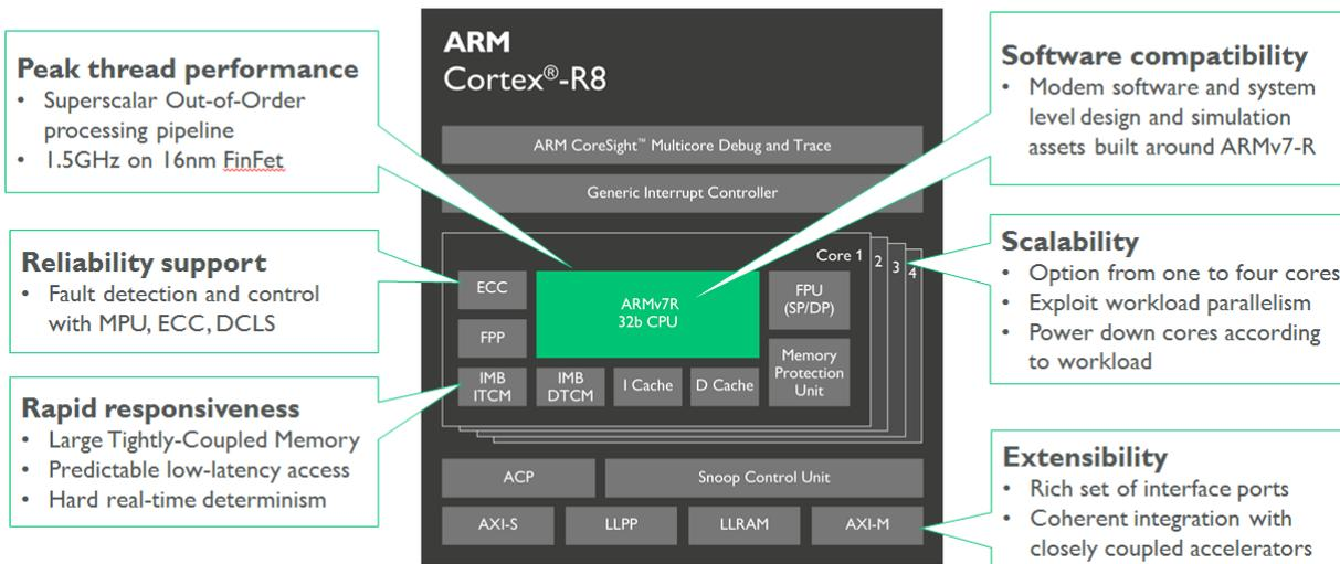
Cortex-R8 also enhances the Tightly Coupled Memory (TCM) to allow more code and data to be held in fast memories, so that there is no delay to access key routines and data. Unlike caches that are managed by the processor, TCMs are managed by the developer so critical instructions and data structures are always immediately available. In modems there are some very critical real-time routines while other routines are less critical and can run in the background.
